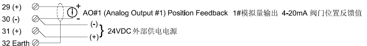
图 3-14 Controlinc 模拟量输出接线 Figure 3 - 14 Controlinc -Analog Output Wiring Connections
